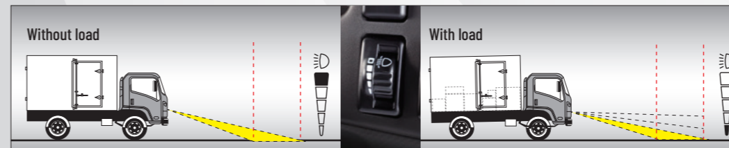
Headlight leveling. Preferred headlight beam position can be maintained when truck is loaded and when it has no load.
